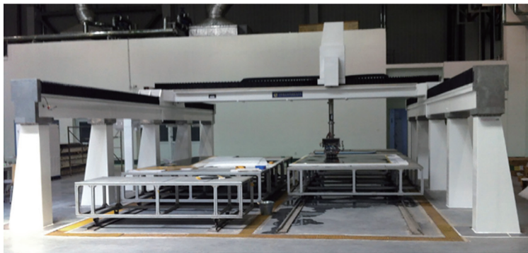
图4 适用于大型航空复合材料翼类结构的CUS-6000 AUT超声检测系统 Fig.4 CUS-6000 AUT system for large aero-composites wing-type structures
